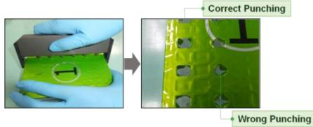
**Fig. 17** Punch the film with the Hole Puncher
