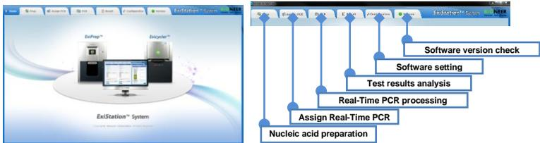
Fig. 8 Tab function of ExiStation™ Manager software
