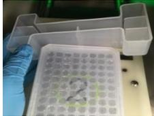
Fig. 25 Loading the Waste tray
