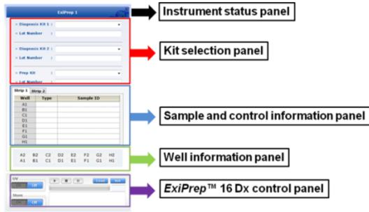
Fig. 10 Prep control panel of ExiStation™ Manager software
