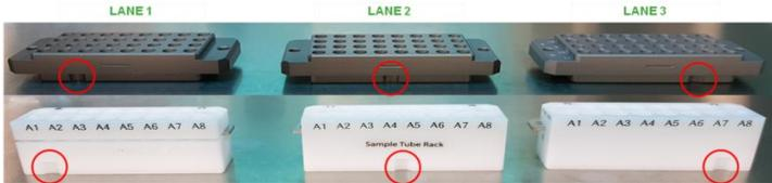
Fig. 61 Checking the position of Elution Tube Rack and Loading Tube Rack
