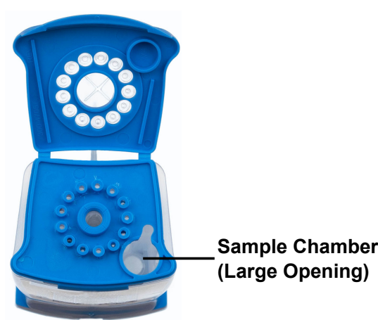
Figure 3. Xpert HIV-1 Qual XC Cartridge (Top View)
