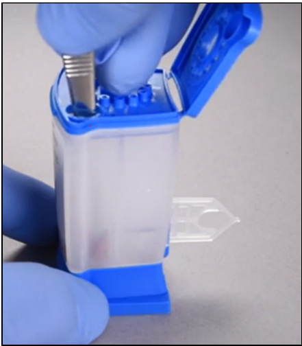
Figure 6. DBS Folded at Bottom of the Sample Chamber
