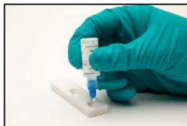
Figure 7. Add Wash Solution vertically.
