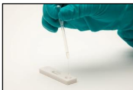
Figure 8. Add sample vertically into device.
