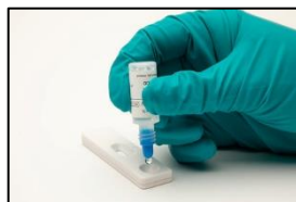
Figure 9. Add Wash Solution vertically.
