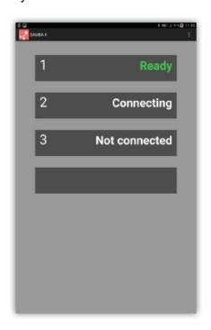
3. If an Assay Module is available, the indicator for the instrument will change from **Connected** to **Ready**. Select button for the Assay Module to proceed with testing.
