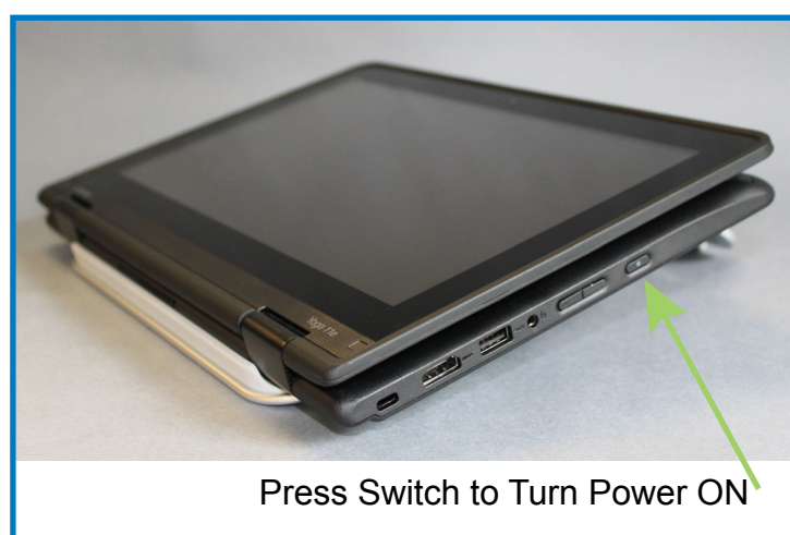
Figure 10. Computer Power Switch
