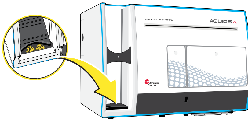
Figure 9.11 Pinch-Point Warning Label on the Autoloader
