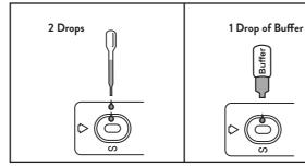
5 Transfer 50 µL serum or plasma or venipuncture whole blood with specimen pipette, then add 1 drop of buffer vertically (approximately 30  $\mu$ L).
