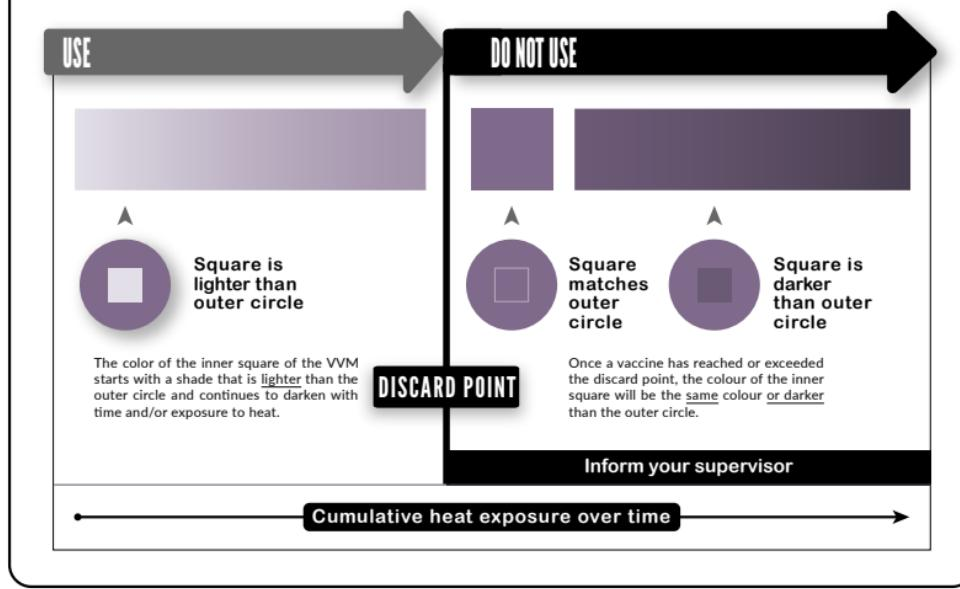
VVM is a label containing a heat-sensitive material which is placed on a vaccine vial/ ampoule to register cumulative heat exposure over time. The colour dot appears on the VVM label in square element is a time - temperature sensitive dot that provides an indication of the cumulative heat to which the vial has been exposed. It warns the end user when exposure to heat is likely to have degraded the vaccine beyond an acceptable level.
