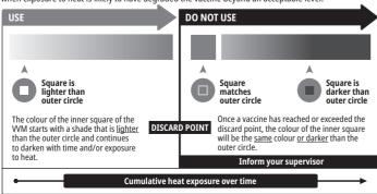
The interpretation of the VVM is simple. Focus on the central square. Its colour will change progressively. As long as the colour of this square is lighter than the colour of the circle, then the vaccine can be used. As soon as the colour of the central square is the same colour as the circle or of a darker colour than the circle. then the vial should be discarded.
