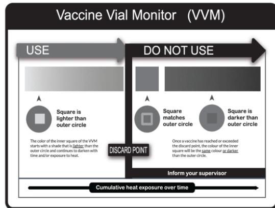
VVM is a label containing a heat-sensitive material which is placed on a Flip-off Seal to register cumulative heat exposure over time. The colour dot appears on the VVM label in square element is a time-temperature sensitive dot that provides an indication of the cumulative heat to which the vial has been exposed. It warns the end user when exposure to heat is likely to have degraded the vaccine beyond an acceptable level.
