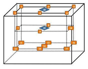
All sensors are to be positioned according to this layout and in direct contact with compartment surfaces.
