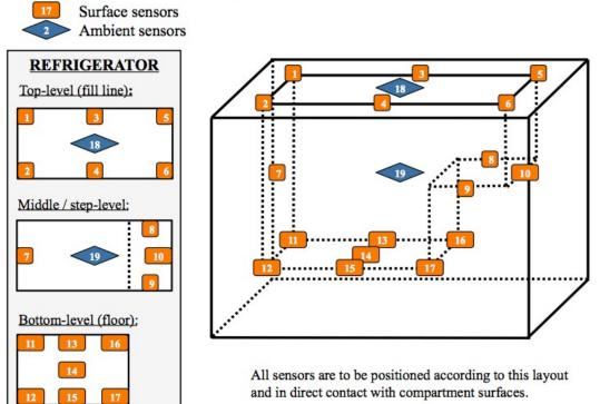
and in direct contact with compartment surfaces.
