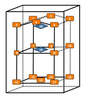
All sensors are to be positioned according to this layout and in direct contact with compartment surfaces.
