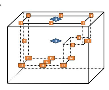
All sensors are to be positioned according to this layout and in direct contact with compartment surfaces.
