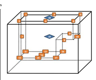
All sensors are to be positioned according to this layout and in direct contact with compartment surfaces.
