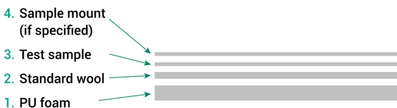
Figure 3. Order of mounting sample – Side view.
