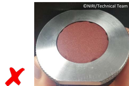
Figure 9. Example of unacceptably mounted sandpaper. Creases are visible around the edge leading to an uneven testing surface (4).
