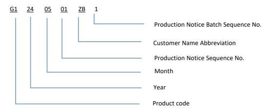
The production batch number for UNET G1 LN products is structured as follows: G1 + Year + Month + Production Notice Sequence Number + Customer Name Abbreviation + Production Notice Batch Sequence Number.
