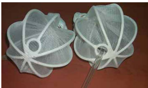
Fig. 1. Wire ball test arena, as depicted in Guidelines for testing mosquito adulticides for indoor residual spraying and treatment of mosquito nets (1)
