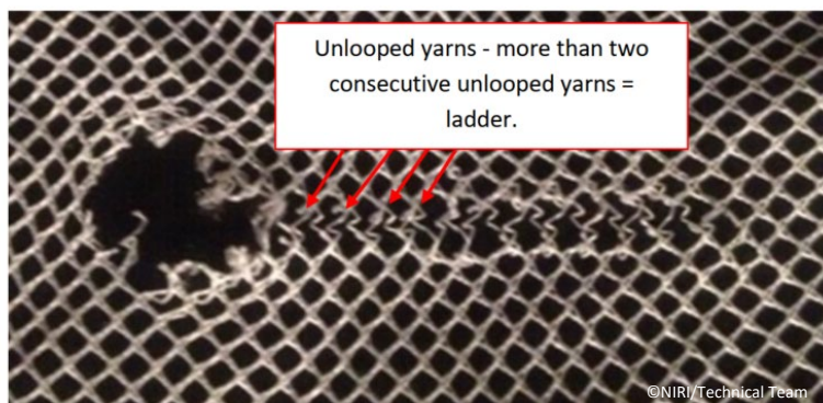
Figure 7. Structure A. Example of laddering. Multiple unlooped yarns are visible - two or more unlooped yarns associated with a ladder.
