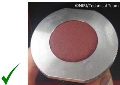
Figure 8. Example of acceptably mounted sandpaper. No creases, flat top (3).
