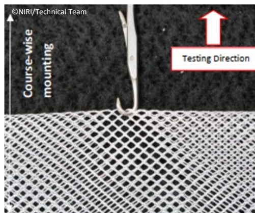
Figure 8b. Example of CW mounting for TESTING in the WW direction.
