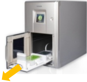
Fig 38. Sliding out the base plate
