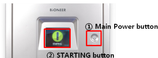
Fig 36. Location of the “Main Power” button and “STARTING” button. on the ExiPrep ™ 16 Dx instrument
