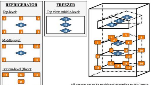
All sensors are to be positioned according to this layout and in direct contact with compartment surfaces.
