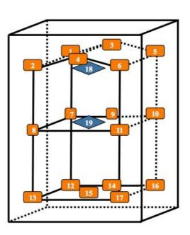
All sensors are to be positioned according to this layout and in direct contact with compartment surfaces.
