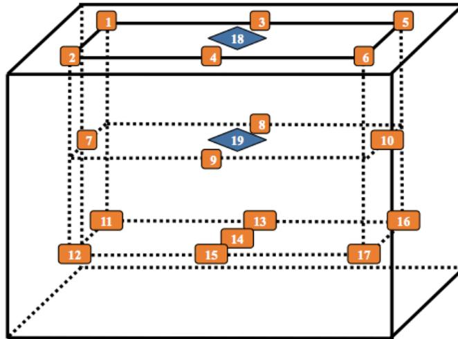
All sensors are to be positioned according to this layout and in direct contact with compartment surfaces.
