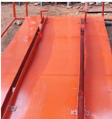
Module to adapt a pick-up truck for patient transport, Democratic Republic of Congo, 2019.
