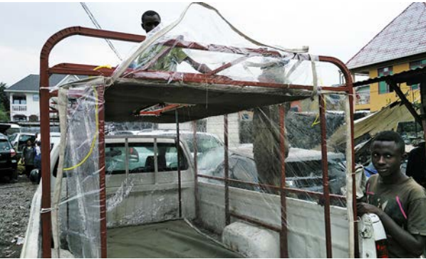
Adaption of a pick-up truck for patient transport, Democratic Republic of Congo, 2019.
