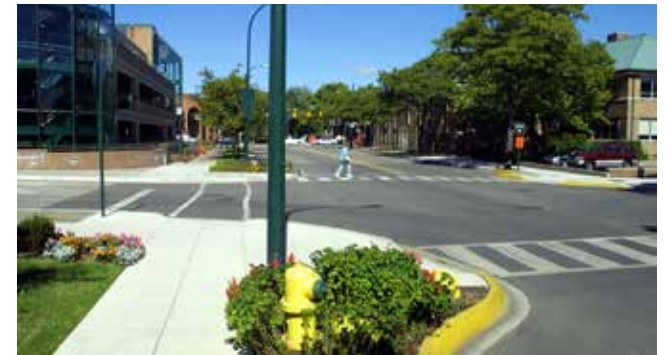
A curb extension in Birmingham, AL shortens the crossing distance for pedestrians
