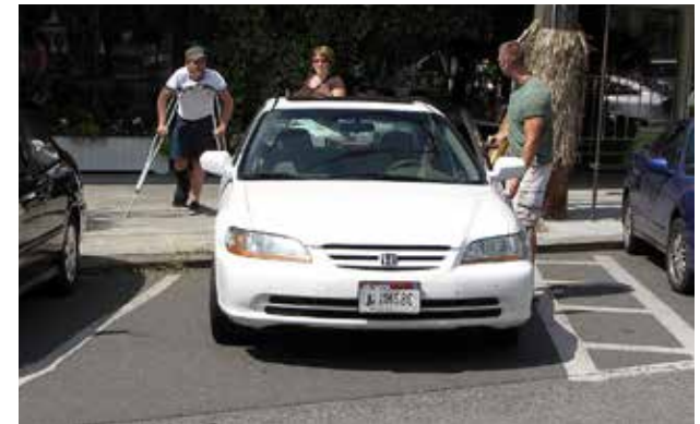
Above: Head-out angled parking is safer for all people, including those driving, biking and walking. Below: This diagram from the City of Northampton, MA illustrates one of the benefits of head-out angled parking: a driver’s ability to see oncoming traffic as they pull into the travel lane from their parking spot.
